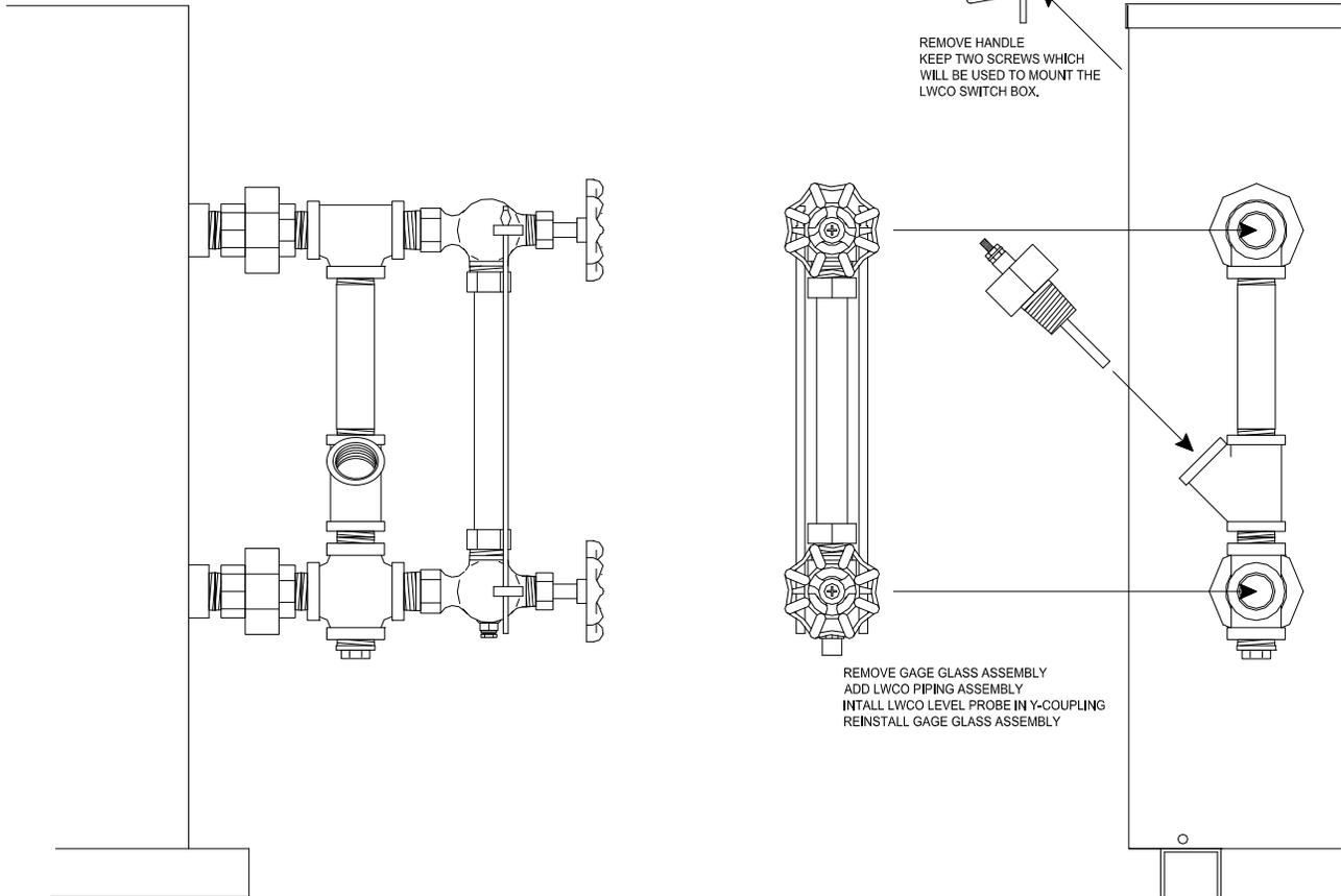
(2) The LWCO is mounted to the boiler's rear panel by removing the handle and using two of the handle screws in the holes provided. *If it is necessary to add a second hole, a 1/8" hole should be drilled 1-1/4" to the left of the lower right handle mounting hole.*
