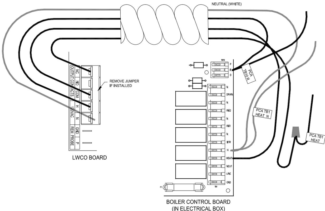
3. Connect the 39 inch black wire to the LWCO's terminal block at the **H** terminal. Run the wire through the conduit. In the electrical box, remove the wire from the circuit board's **R** connection in the small terminal block then twist that wire's end together with the black **H** wire from the LWCO and reinsert the twisted wire ends into the circuit board terminal block's **R** connection.
