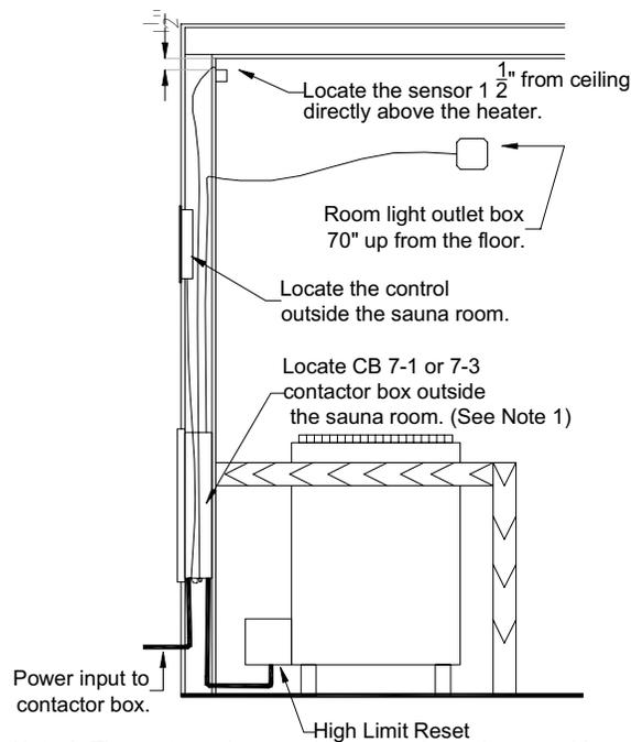
**Note 1:** The contactor box may be mounted anywhere outside the sauna room. A location should be selected so the front cover is accessible for service and the noise of the contactor pulling in will not be a nuisance.
